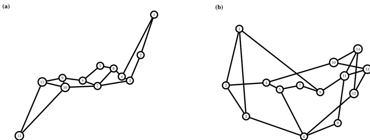
Fig. 3. Simulated network topologies: a) Japan Photonic Network (JPN12); b) National Science Foundation Network (NSFNET).
