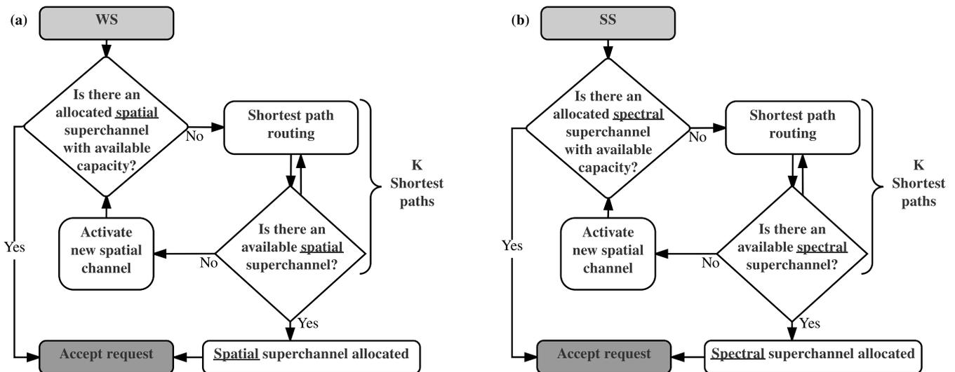
Fig. 2. The resource allocation algorithms are shown in (a) for WS, and (b) for SS.
