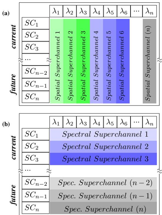
Fig. 1. Current and future example of link occupation with (a) wavelength switching of spatial superchannels and (b) full-spectrum spatial switching. In the figure,  $SC$  denotes spatial channel and  $\lambda$  denotes wavelength channel.
