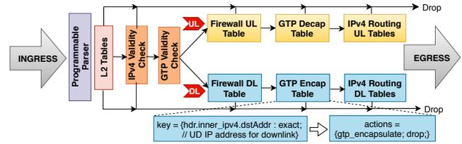
Figure 4: P4-defined vEPG pipelines featuring the main Up-link (UL) and Downlink (DL) tables
