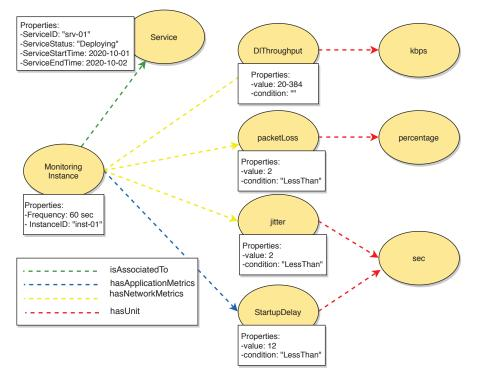
Figure 8 Instance of Monitoring model generated automatically by the MMG component using 3GPP IM.
