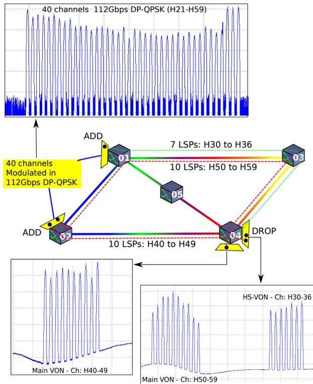
Fig. 8. Optical Spectrum at nodes 01, 02 and 04
