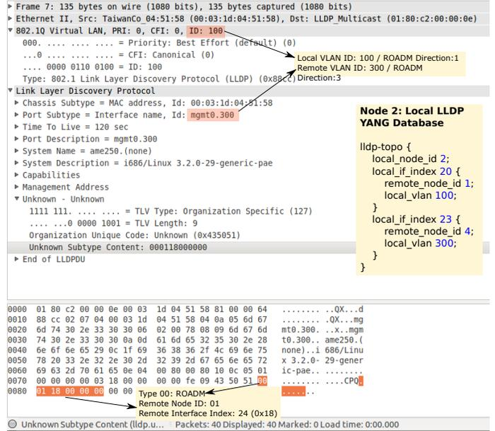
Fig. 4. LLDP packets and YANG Topology Database
