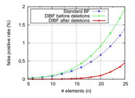
Fig. 4. Observed average fpr of a 240-bit DlBF with r = 24 and k = 5, before and after removing elements, compared to a 240-bit SBF.
