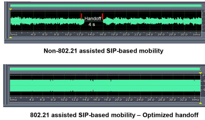
Figure 4.3: Optimized SIP based mobility assisted by 802.21 by reducing the disconnection time [DOea].
