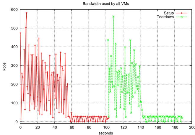
Fig. 8. Control Traffic between XCP-V plane and real nodes for establishment and removal of 27 lightpaths
