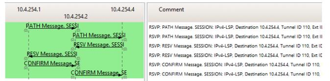
Fig. 6. RSVP messages during LSP establishment
