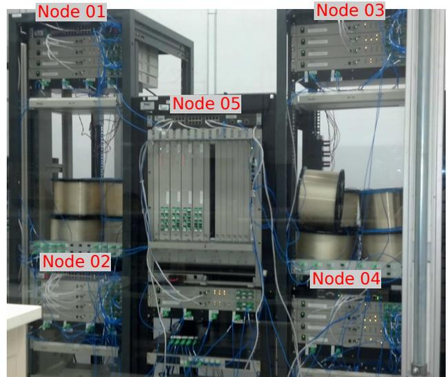
Fig. 2. Testbed composed by five WSS ROADMs
