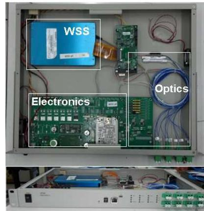
Fig. 3. Testbed WSS ROADMs line card
