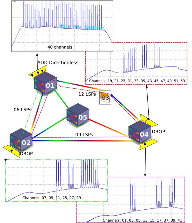
Fig. 7. Optical Spectrum at nodes 01, 04 and 03
