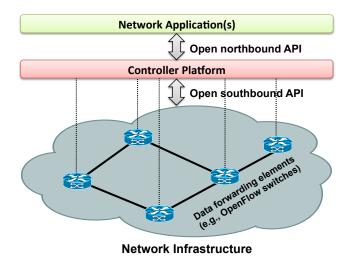
Fig. 1. Simplified view of an SDN architecture.
