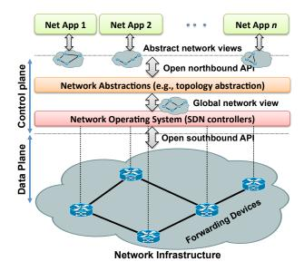
Fig. 4. SDN architecture and its fundamental abstractions.
