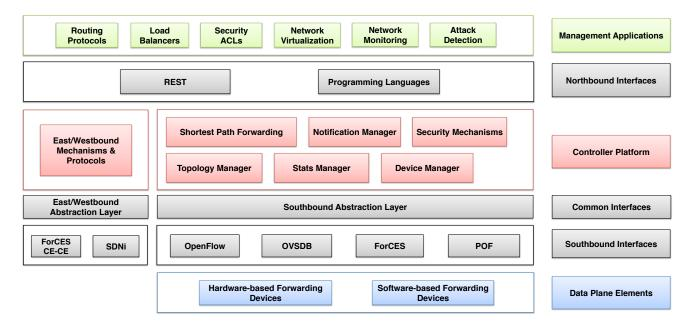
Fig. 8. SDN control platforms: elements, services and interfaces
