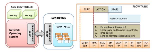
Fig. 7. OpenFlow-enabled SDN devices
