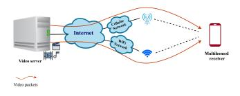
Figure 3: Multipath wireless video streaming over LTE and WiFi networks.
