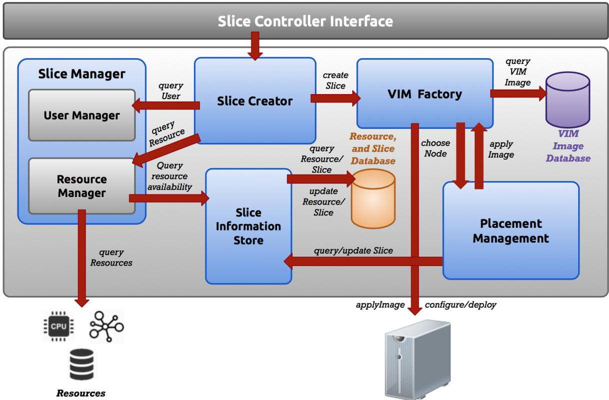
Fig. 4. DC Slice Controller Architecture
