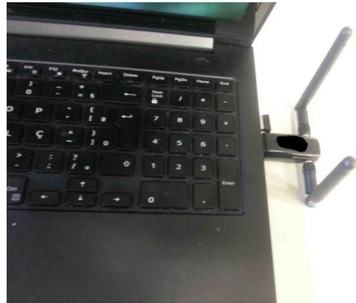
Fig. 4. Physical wireless NIC integrated into Mininet-WiFi.
