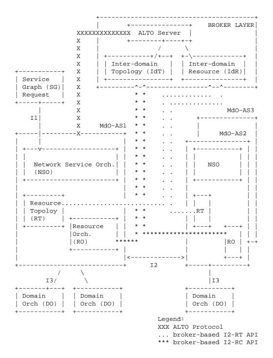
Figure 2: Broker-assisted 5GEx Info Exchange
