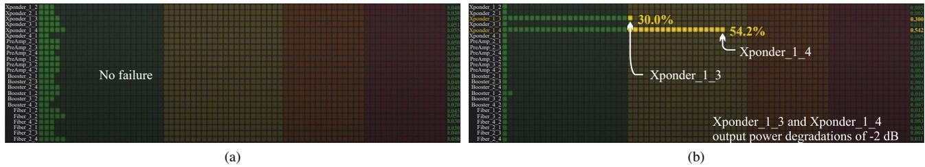
Fig. 6. Probability bar graph of the ANN output displayed with Grafana. In this example, we introduce a 2-dB output power degradation at Xponder\_1\_3 (transponder located at node N1 that communicates with node N3) and Xponder\_1\_4 (transponder located at node N1 that communicates with node N4). (a) ANN output before the failure. (b) ANN output after the failure, indicating an empirical probability of 30.0% (Xponder\_1\_3) and 54.2% (Xponder\_1\_4).
