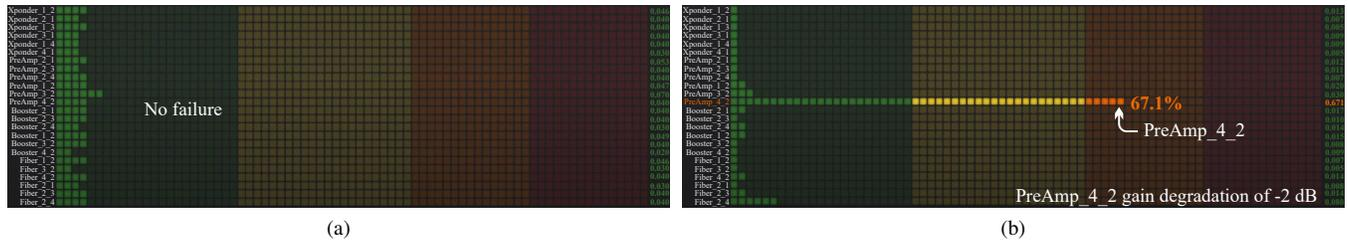
Fig. 4. Probability bar graph of the ANN outputs displayed with Grafana. In this example, we add an artificial 2-dB gain degradation to PreAmp\_4\_2 (preamplifier in the link interconnecting nodes N2 and N4). (a) ANN output before the failure (b) ANN output after the failure (67.1% empirical probability).
